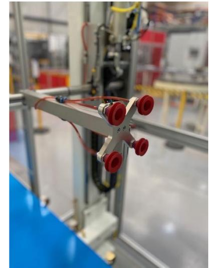
A vertical take-off transfers moulds from the Injection Mould Machines, rotates 90 degrees and sets product onto a conveyor, where product can be indexed, or collated into stacks, via servo motion.
